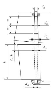
Fig. 3.4.1. Required rudder stock diameters
