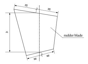
Fig. 3.2.1. Determining of the rudder blade height
