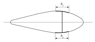
Fig. 3.5.2.5. Streamline rudder blade section with girder applied
