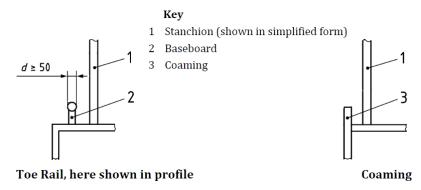
Fig. 11.1.1. Guard rails in way of deck edge
