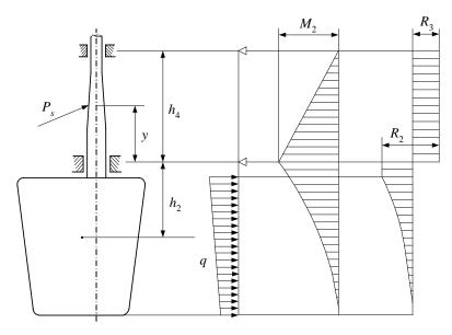
Fig. 3.2.3.3 Underhung rudder
