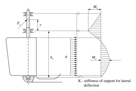
Fig. 3.2.3.2. Supported rudder
