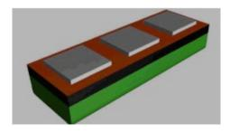
(2) Detached hatchways connected by longitudinal coamings.
