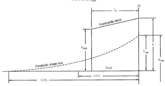
The height of the forecastle at the bulkhead position shall not be less than the ordinate, at that point, of a parabolic sheer curve having an ordinate  $S_{\min}$  at the forward perpendicular and extending aft for a distance of 0.15L from the forward perpendicular.
