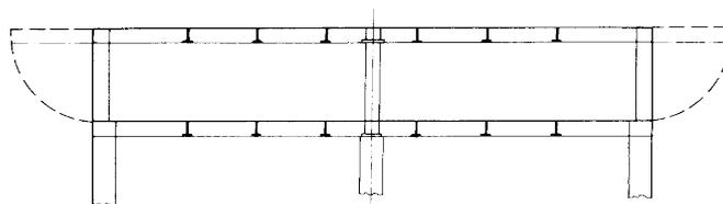
b) Grillage model (upper deck), including ship sides unfolded
