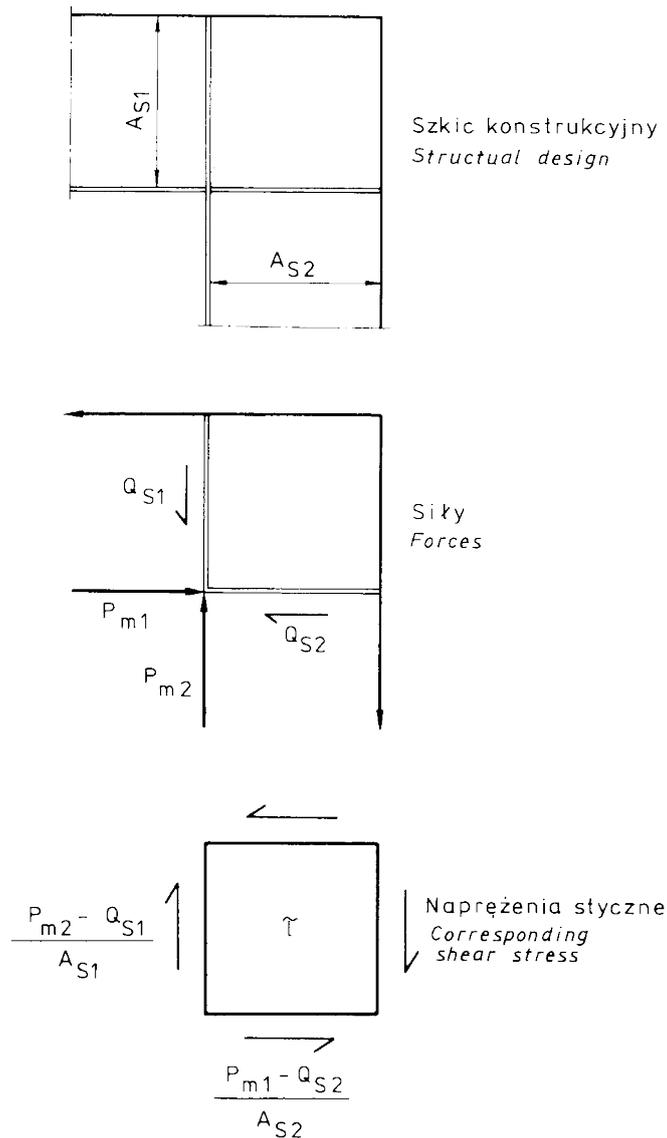
Fig.4.2-1 Stress analysis of cross joint
