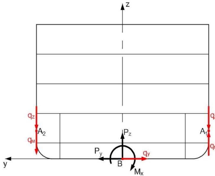
Fig. 5.3-1 Balance method for FE model of the whole ship hull
