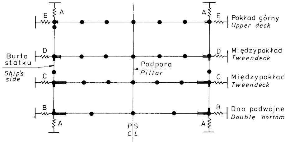
Fig.3.2-1 Transverse web frame at pillars
