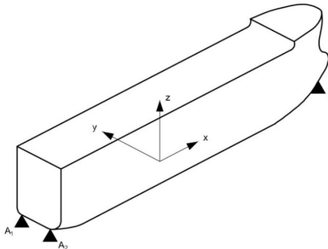
Fig. 5.3-2 Fixed supports in FE model of the whole ship hull
