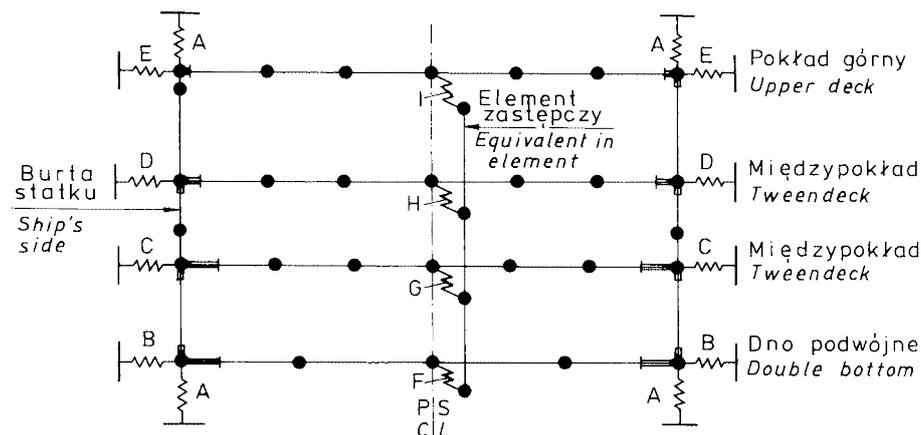
Fig.3.2-2 Transverse web frame between pillars
