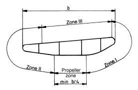
Fig. 11.5.2.1 Longitudinal section through nozzle ring
