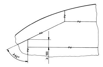
Fig. 3.3.1 Arrangement of welded joints
