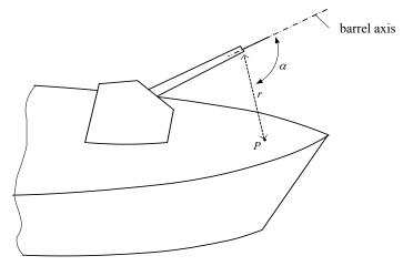
Fig. 5.3.3 Parameters for pressure  $p_z$  calculations
