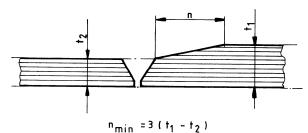
Fig. 4.2.1.2 Edge preparation for welding plates of different thickness
