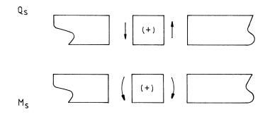
Fig. 15.4.2 Positive sense of bending moments and shear forces
