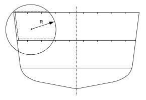
Fig. 6.2.1 The hull damaged region due to projectile explosion inside the ship
