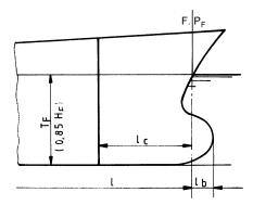
Fig. 9.2.2.1 Position of collision bulkhead
