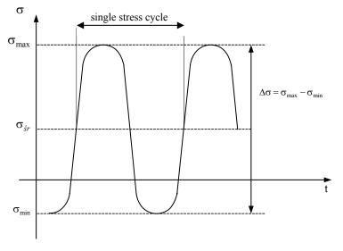
Fig. 16.2.3 Definition of stresses cycle and the range of stresses
