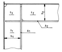
Fig. 13.8.3.5 Bracketless connection of girders
