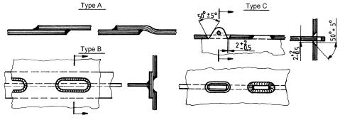
Fig. 4.2.2.1 Lap and slot welds
