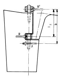
Fig. 11.3.2-2 Forces in semi-spade rudder
