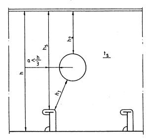
Fig. 3.2.3 Determining the net web height
