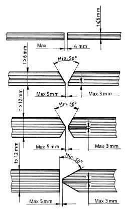
Fig. 4.2.1.1 Edge preparation for manual butt welding
