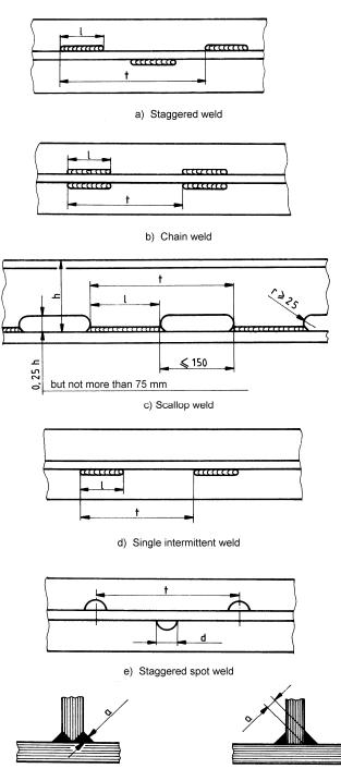
f) Thickness a of fillet weld
