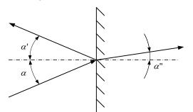
Fig. 4.3.4.1 Reflection and refraction of the underwater shock wave on the media border
