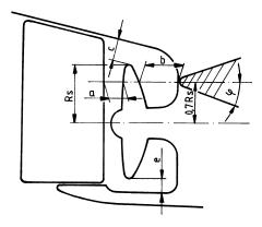
Fig. 11.4.2 Propeller clearance
