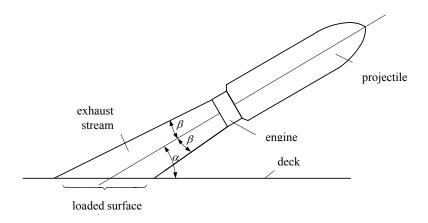
Fig. 5.4.1 Load from the exhaust stream
