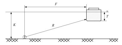
Fig. 4.3.2.1 The distances for impact number estimation
