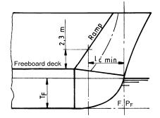
Fig. 9.2.2.3 Collision bulkhead with a ramp
