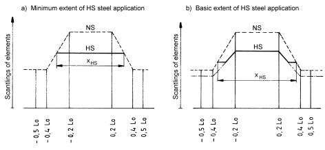
Fig. 15.6.2 Longitudinal extent of HS steel
