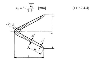
Fig. 11.7.2.4 Cast sternframe propeller post
