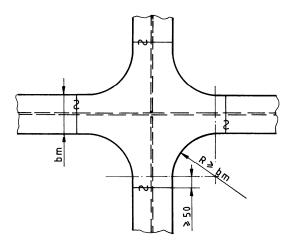
Fig. 3.3.2 Joints of girder face plates
