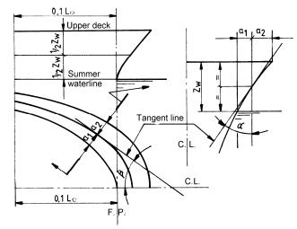
Fig. 7.4.5 Side plating flare angle
