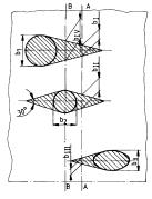
Fig. 15.7.2.2 Examples of determining the influence of openings on the effective sectional area
