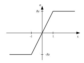
Fig. 2.2.3 Dependence  $\sigma - \varepsilon$  for elastic-plastic strains
