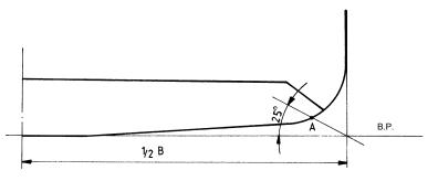
Fig. 6.1.2.4 Overlapping the bilge by the margin plate
