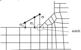
Fig. 14.7.5.1 Principle of stresses values extrapolation
