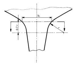
Fig. 11.3.6 Transition zone between rudder horn and hull plating
