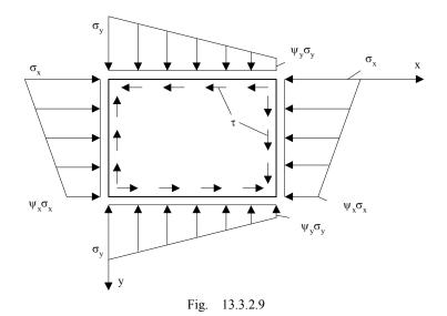
**13.3.2.10** Stress values applied in evaluation of buckling strength of a construction, in cases other than those specified in 13.3.2.7 and 13.3.2.8, are to be calculated within zone strength analysis of the construction according to the provisions of Chapter 14.
