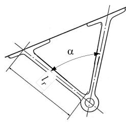
Fig. 11.6.3.8 Double-arm strut
