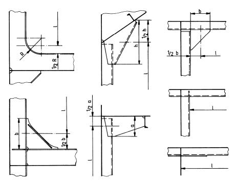
Fig. 3.2.1.1 Determining the span of structural members
