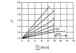
Fig. 6.2.3.3-2 Dynamic factor for spur gear. Accuracy classes 3 ÷ 8 acc. to ISO 1328
