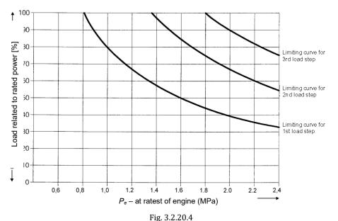
Limiting curves for loading 4-stroke engines step-by-step from "no load" to rated power as the function of brake mean effective pressure  $P_e$ , [MPa]
