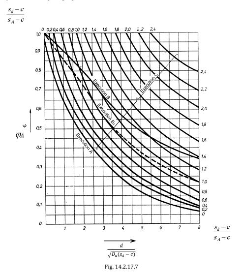
**14.2.17.8** Where disc-shaped plates are used to strengthen openings in cylindrical, spherical or conical walls, the dimensions of the strengthening plates shall be determined in accordance with the following formulae:
