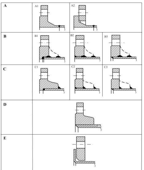
Table 15.3.2.3Acceptable types of flanges for piping connections
