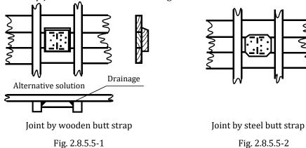
Wooden butt strap thickness shall be equal to the planking thickness. Steel butt strap thickness shall be equal to 15 - 18 per cent of the planking thickness. The minimum number of metal bolts or rivets for one side of the joint is:
