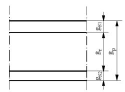
$g_r$  - core thickness, [mm],  $g_{s_1}, g_{s_2}$  - cladding thickness, [mm],
