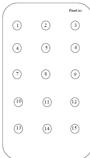
Figure B-2 Thickness measurement locations
