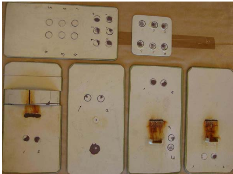
Figure C-1 Overview picture of the panels after exposure in the wave tank and the heating chamber. Reference panel not exposed – top right. Picture taken after examination (example picture not connected with example results in this model report).
