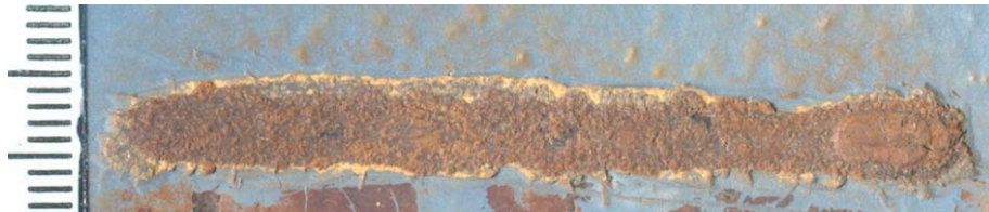
Figure C-6 Undercutting from scribe, side wave tank panel with cooling (example picture not connected with example results in this model report).
