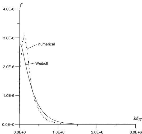
Fig. 10. The difference between numerical and Weibull distribution of hull girder wave bending moment
