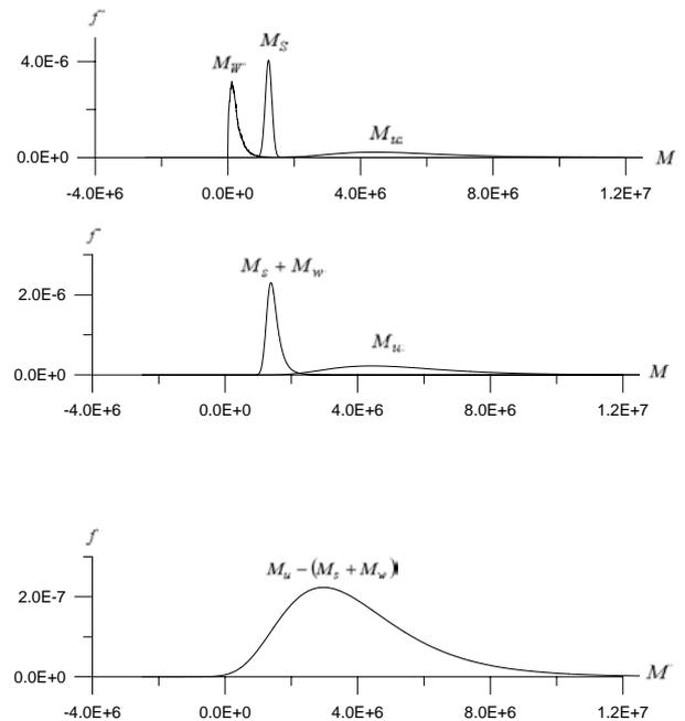
Fig. 8. The probability distributions of hull girder strength
