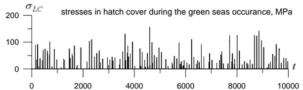
Fig. 7. Time history of stresses in the hatch cover caused by green seas
