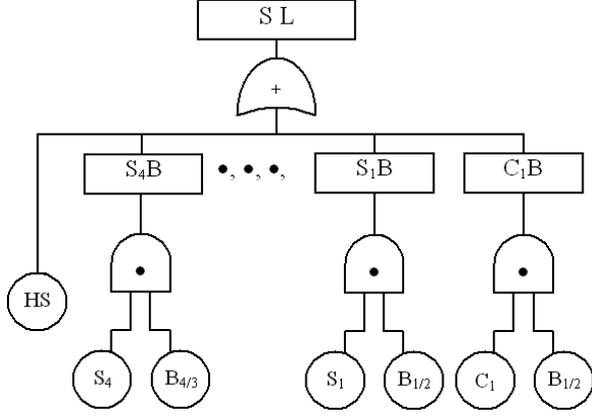
Fig. 1. Simple fault tree of bulk carrier structure failure
