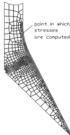
Fig. 5. Point of the frame in which the greatest stresses occur
