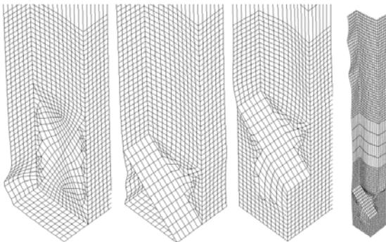
Fig 6. The destroyed bulkhead single corrugation
