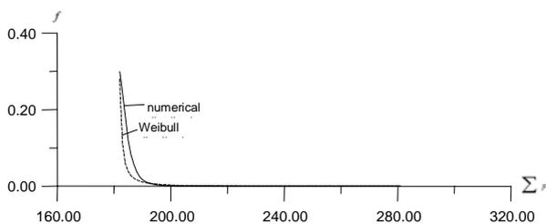
Fig. 11 The difference between numerical and Weibull distribution of frame stresses
