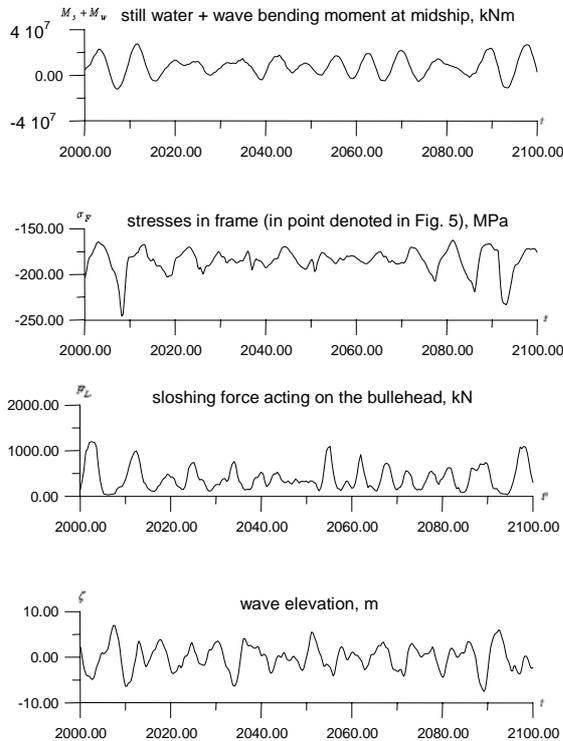
Fig. 4. Time history of: vertical bending moment  $M_S+M_W$  in the midship of hull, stresses  $\sigma_F$  in the side frame of hold No 4, perpendicular to the bulkhead sloshing force  $F_L$  acting on one corrugation of the bulkhead and the wave elevation
