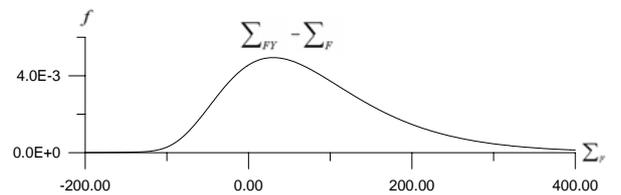
Fig. 9. The probability distributions of frame strength (in way of hold No 4)
