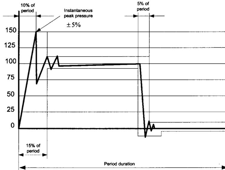
Fig 2.3.1 Impulse pressure diagram
